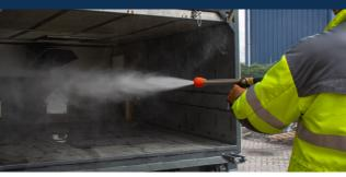
> The new spray gun now has two spray settings: a very powerful jet stream, and a wide-spread fan pattern that covers a larger area with greater efficiency. With this new high-pressure spray gun, operators can quickly and easily clean the sweeper and street furniture like bins and bus stops.
