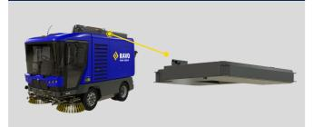
An extra roof mounted 420-litre tank will give the sweeper a class leading total water capacity of over 950 litres without taking hopper space away. This enables a longer operating time between water refills, keeping the sweeper on the streets and on the go.
